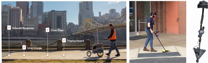
Left: technician collecting sidewalk measurements while using pathMet; Center: technician collecting curb ramp data using curbMet; Right: curbMet
