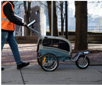
Left: technician collecting sidewalk measurements while using pathMet; Center: technician collecting curb ramp data using curbMet; Right: curbMet
